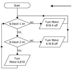
This flowchart could be one version of a line follower. The light sensors inputs 1 and 2 would have to be on either side of a dark line. It might be an
