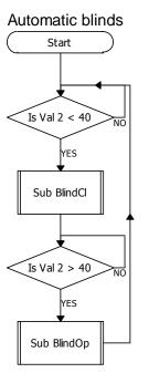
Activity 4: First build two subroutines, BlindCl and BlindOp, which make Motor B go forward and reverse [similar to the Barrier example earlier].
