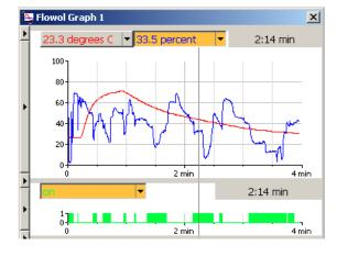
The vertical cursor line can be dragged across the graph to scan the values at the various times.
