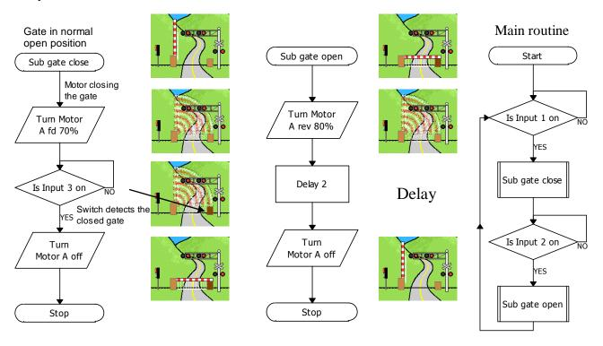
When using this 2D barrier mimic, you need to click on the gate post 'hot spot' to simulate input 3 being turned on. When the barrier opens however, this switch will 'spring' off automatically.
