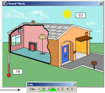
In the mimic shown: Val 1 is the outside temperature reading and Val 2 the outside brightness.
